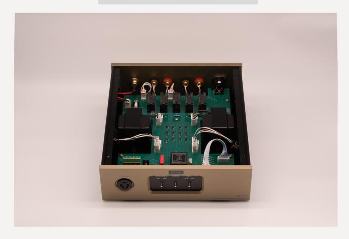
Gain (8  $\Omega$ ): 31.1 dB Gain (16  $\Omega$ ): 27.8 dB
